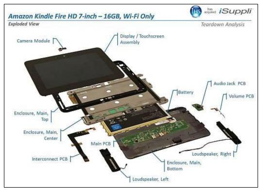
Components i Hardware Elements Retail Pricing (As of November 2012) **Total BOM Cost** Manufacturing Cost BOM + Manufacturing Major Cost Drivers Memory: 1GB LPDDR2 + 16GB eMMC NAND Flash + DRAM Display & Touchscreen: 7" 1280x800 w/ Multitouch Processors: TI OMAP4460BCBS Camera(s): 1MP 720p BSI User Interface & Sensors & Combo Module (WLAN/BT/FM) Power Management Battery: 3.7V 16.4Wh Li-Polymer Mechanical / Electro-Mechanical / Other **Box Contents** Source: IHS iSuppli Research, November 2012
